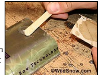
Filling the screw hole with epoxy.
