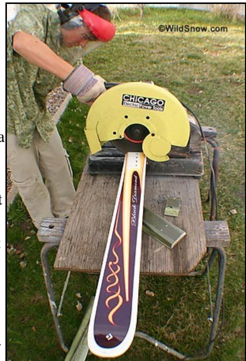
The ultimate coreshot. Cutting a Black Diamond Crossbow ski in half for testing.
